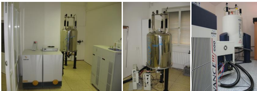
Obr. 4.19 - Varian NMRS 300 MHz, Varian INOVA 400 MHz, Bruker Avance III 600 MHz
